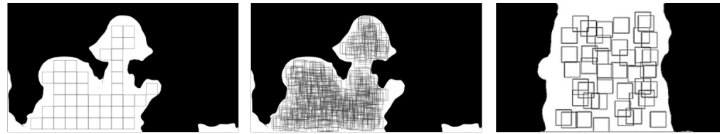
(a) Foreground Unique Patch Sampling (b) Foreground Random Patch Sampling (c) Foreground Jitter Patch Sampling
